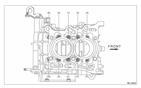
(10) Install the upper bolt to cylinder block.
